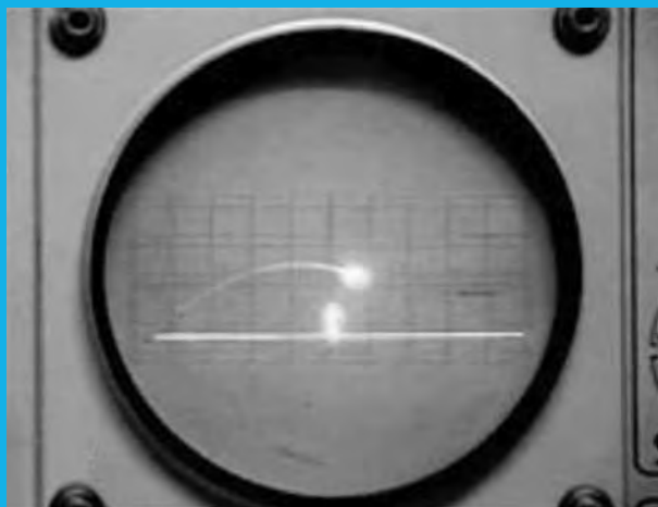
FIGURA 3: TENNIS FOR TWO RODANDO NO OSCILOSCÓPIO DO BROOKHAVEN NATIONAL LABORATORY.
